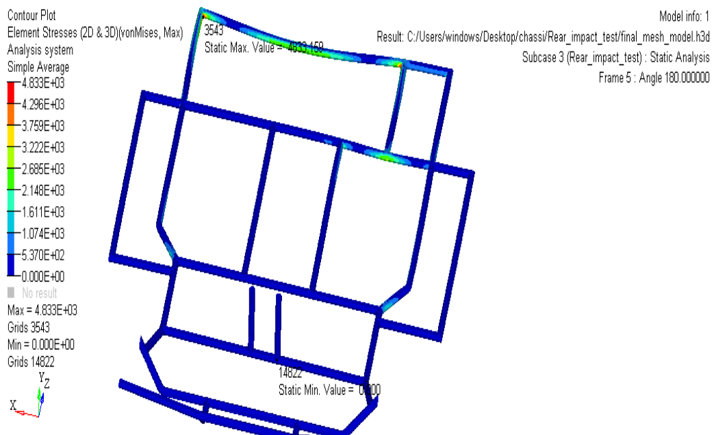
Fig. No.9. Stress Plot for Rear impact Test
